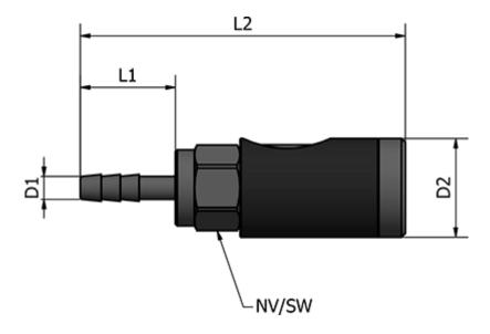
D1 ((mm) = Ø13 D2 (mm) = 26 L1 (mm) = 25 L2 (mm) = 88.5 SW (mm) = 21 Weight (g) = 121
